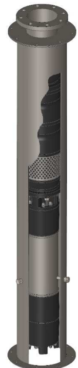
Figure 1 : Correct installation of the submersible electro-pump inside a well without cooling sleeve
